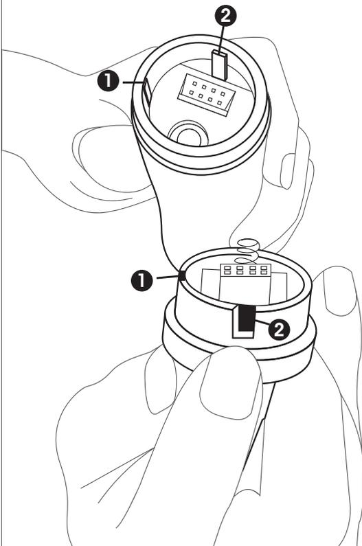
1. Align the corresponding position with the checkpoint
