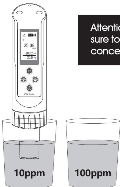
**Attention: Before calibration after activation, please make sure to thoroughly clean the electrode and calibrate from low concentration to high concentration.**
